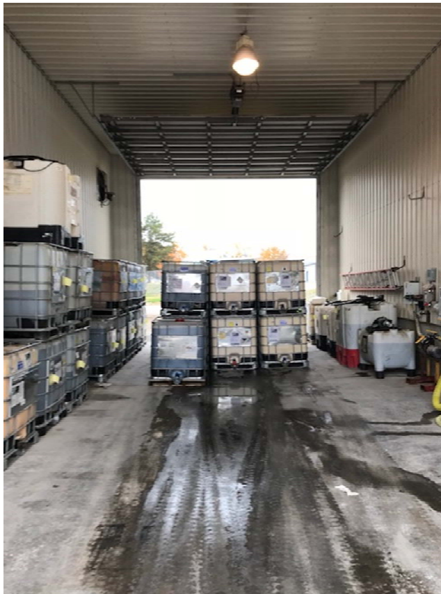
Fig. 6) Mini-bulks moved into a contained area.
