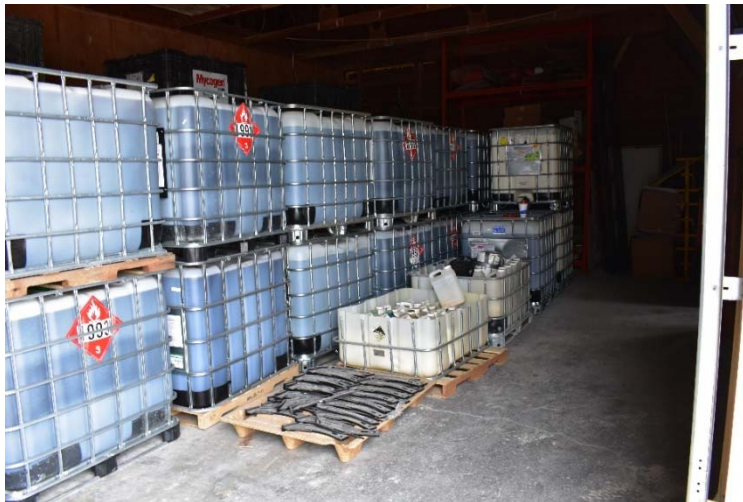
Fig. 1) Mini-bulks being stored out of containment.
